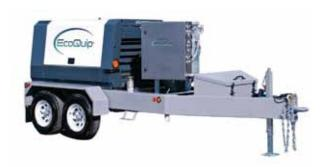
Engine: 4-cylinder Turbo Diesel 45~57 HP @ 2600RPM Battery: 12 Volt Operating Pressure: 100 psi (7 bar)
