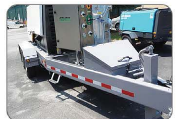
Tandem axle trailer with integrated water tank, storage box, and heavy duty jack stand.
